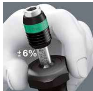
Measurement accuracy is ± 6 % (article 1430: ± 10 %) in accordance with the standard DIN EN ISO 6789. Distinctly audible and noticeable excess-load signal when the pre-set torque is reached.
